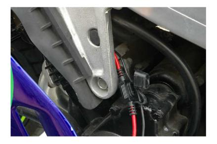
If needed, you can remove the fuse to make it easier to feed the cable through tight spots. Alternatively, loosen the front and rear tank bolts.
