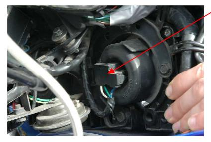
Pull the connector off the bulb.
