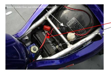
Bolt the O-Ring terminals to the battery terminals.
