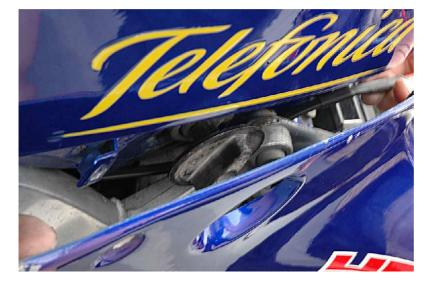
Feed the end with the ring terminals under the frame and along side the tank, through to the battery
