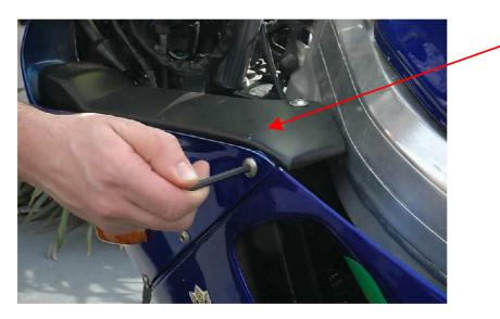
Remove the air duct.
