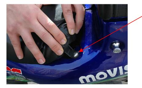
Peel back the rear corners of the seat padding and unscrew the two bolts.
